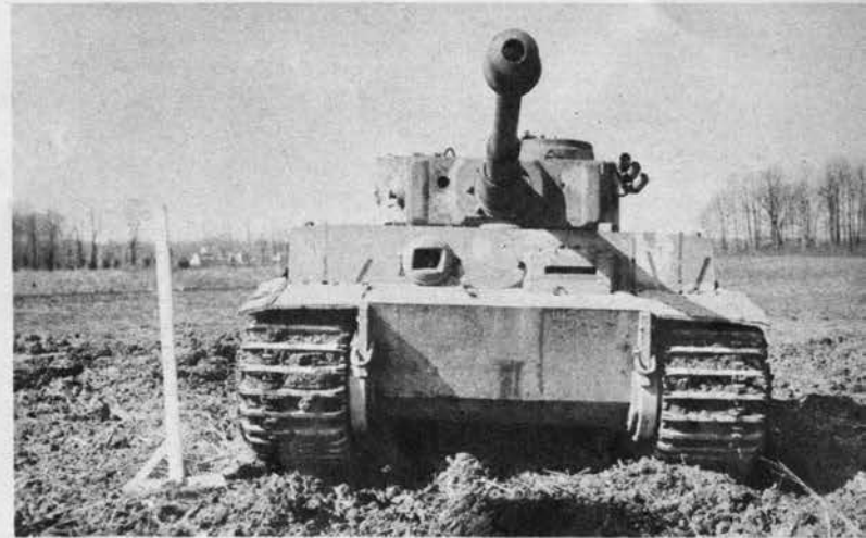
Tiger is impressive in head-on view. Long-barreled gun with large muzzle brake points from the broad flat face of forward-sitting turret. The prominent cupola is offset to the left and rear.
